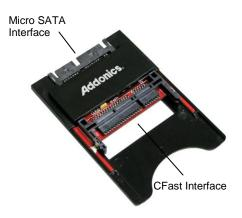
The Micro SATA CFast adapter enables using of CFast media as a replacement for the Micro SATA hard drive in the iPOD or the sub-Notebooks. Once installed, the CFast media behaves like the Micro SATA SSD with low power consumption, fast access time and completely shock resistant.
